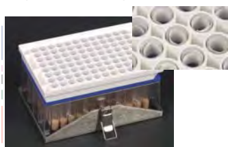
Figure 1: MicroResp™ measures the community level physiological profile of the microbial community as the response to various additions of chemically different types of radiolabelled carbon as respired C14-CD 2 trapped in alkaline.
