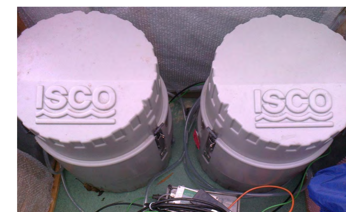
Teledyne ISCO 6712 automatic samplers at gauging station
