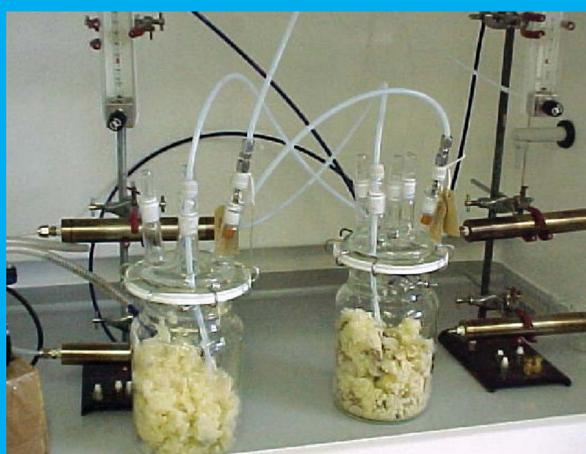
The volatile chemical compounds released by the cooked potatoes were collected and then analysed by Gas Chromatography - Mass Spectrometry (GC-MS) in order to identify them. A large number of compounds have been identified in boiled potatoes. Several of
