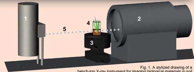
Fig. 1. A stylized drawing of a bench-top X-ray instrument for imaging biological materials in soil showing: 1) the source of X-rays, 2) the detector, 3) the rotating turntable, 4) the soil microcosm and plant/insect, and 5) the path of the X-ray beam
