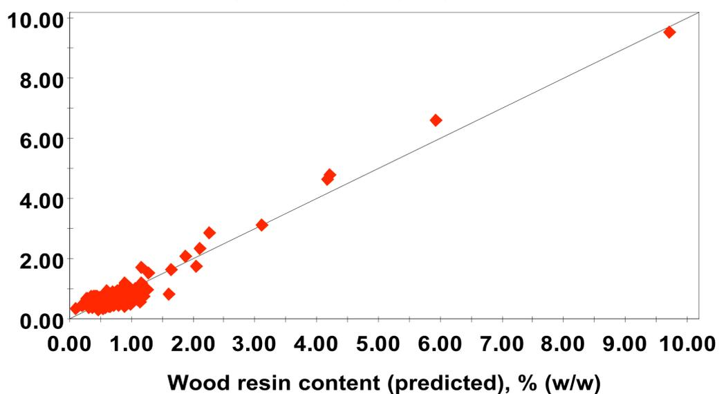
**Fig.4.** DRIFT based model for prediction of resin content of wood.
