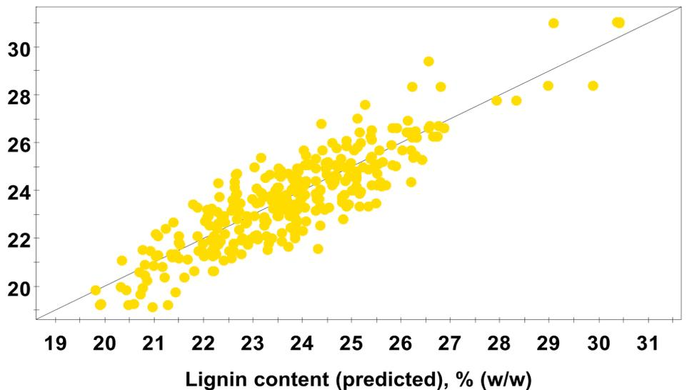
**Fig.3** Calibration between measured and predicted lignin content on the basis of DRIFT spectra.
