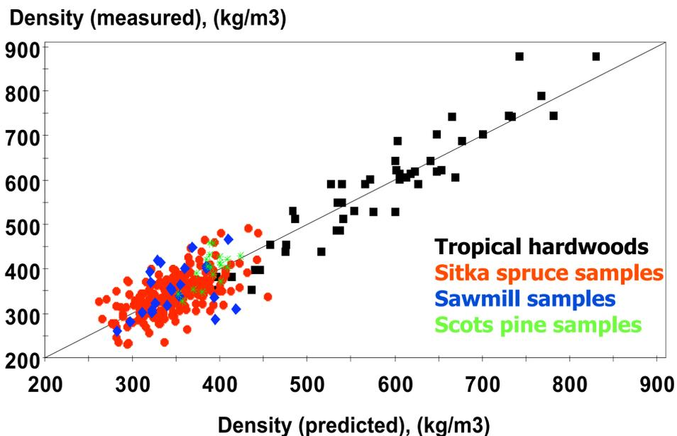
**Fig.1** Calibration between wood density and FT-IR spectral data.
