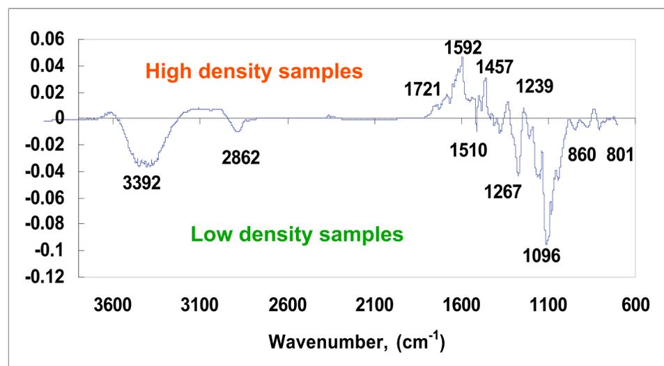
**Fig. 2.** PLS regression coefficients of the density model showing spectral differences due to density variation.
