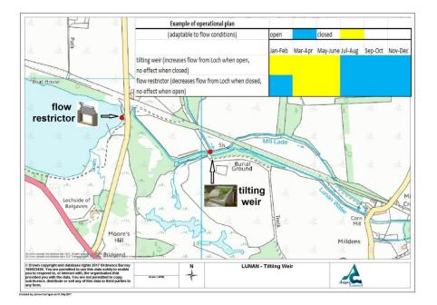
Figure 1. Potential location of proposed hydraulic structures at the outlet to Balgavies Loch, to provide improved water management. The line along the north shore of the lade shows the main proposed area for dredging.
