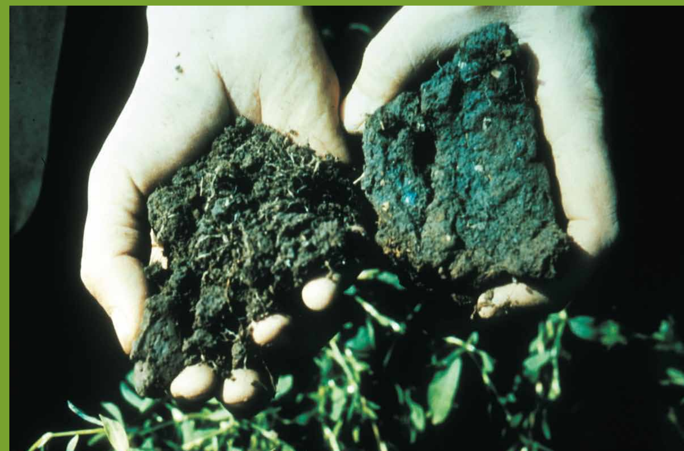
Soil clod on right is compact due to continual traffic, blue-grey in colour due to reducing conditions and poor environment for root development. Soil clod on left is relatively loose, ample pore space for good, healthy root development.
