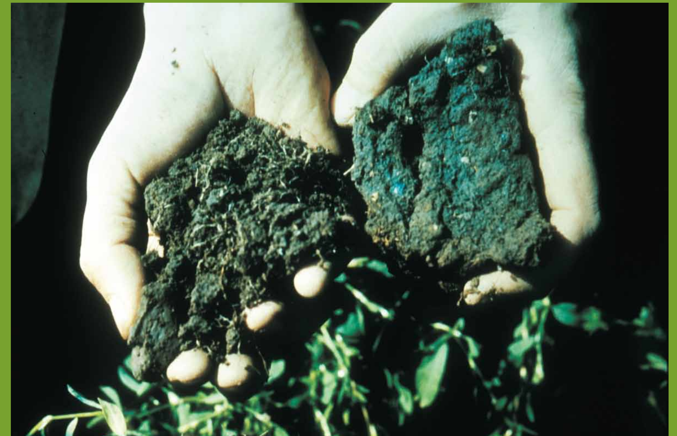
Soil clod on right is compact due to continual traffic, blue-grey in colour due to reducing conditions and poor environment for root development. Soil clod on left is relatively loose, ample pore space for good, healthy root development.
