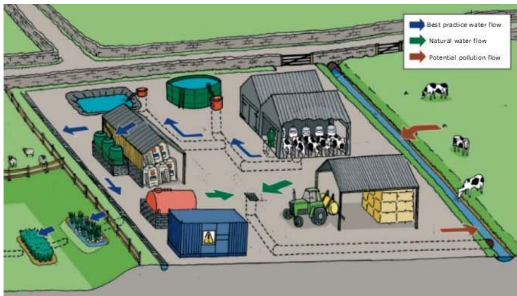
Figure 3: Water flow around the farm showing potential pollution flow (brown arrows), best practice flow (blue arrows) and natural flow (green arrows), after DEFRA, (2012) and Environment Agency, (2007).
