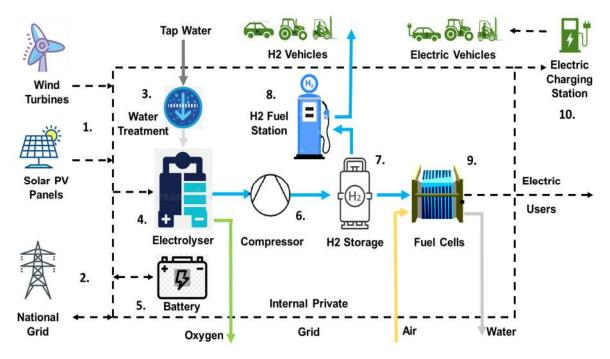
*Component 1. Renewable power generators.* The most abundant renewable-power resource at Glensaugh was determined by RINA to be wind, followed by solar. The solar profile is seasonally out of phase with peak demand (winter), but solar PV can act as a 'top-up' to balance generating capacity at times when the wind turbine is working at reduced capacity.
