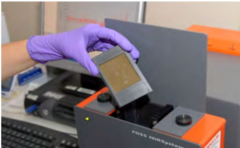
Fig. 1: Soil sample analysis using a NIR spectrophotometer
