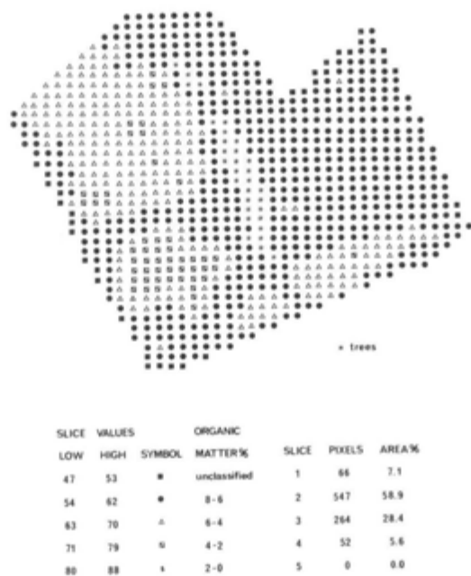
Fig. 2.3b. Surface soil variation (soil organic matter) classified using airborne multispectral scanner data.
