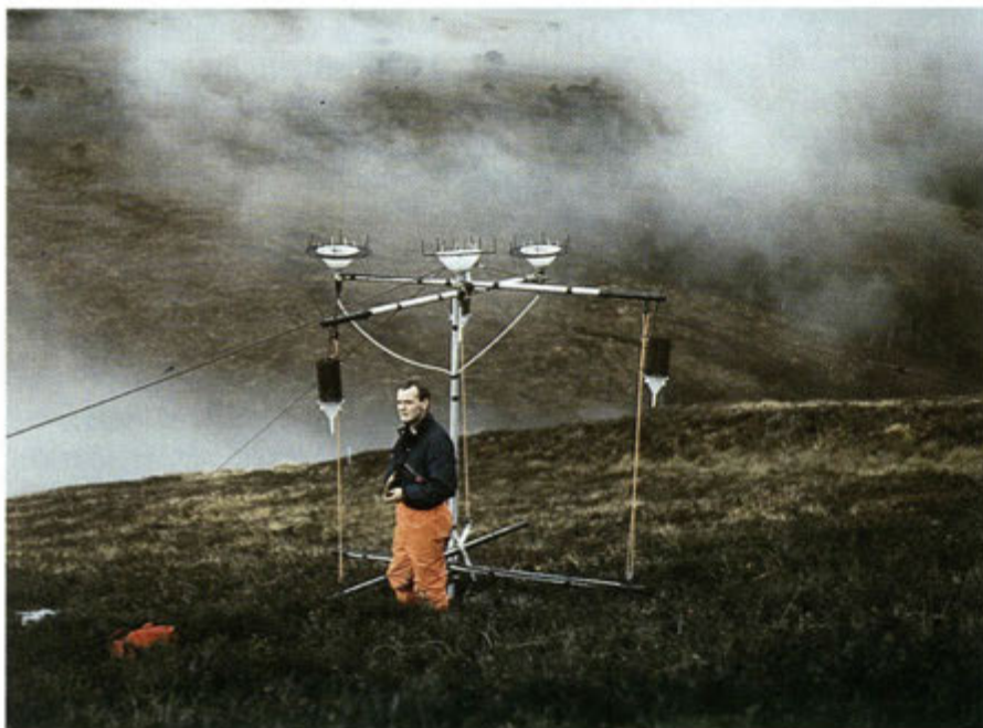
Figure 3. Input monitoring assembly at Allt a'Mharcaidh. The larger white funnels are nipher-shielded bulk precipitation collectors, while the smaller interception gauge funnels (shown at a larger scale on the right) have a coarse mesh superstructure to enhance the trapping of mists and other aerosols.
