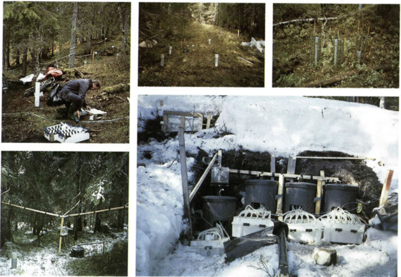
Figure 1. The experimental equipment (bottom right) installed on the SWAP sites is capable of sampling all of the available water passing into, and through, the system. All parts of the plot systems (inputs, throughputs and outputs) can be connected to event samplers, which provide synchronous discrete water samples. Here the drainage from four different soil horizons in a soil pit at Høylandet is being collected during the first soil water throughflow after snowmelt in 1987.
