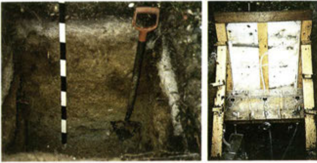
Figure 2. Soil water throughflow is collected from a vertical soil face, as exposed in the pit at Høylandet (left). Water is sampled at the different levels, or horizons, of the soil and volumes are measured by passing the separate drainage tubes into tipping-bucket gauges mounted in front of the completed assembly shuttered framework backfilled with inert polythene beads (right).
