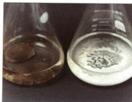
Figure 7. Solubilization of iron phosphate (after 6 weeks incubation at 25^\circ\text{C} ) by an unidentified fungal species (in flask to left of photograph). Flask to right of photograph, with iron phosphate but not inoculated.
