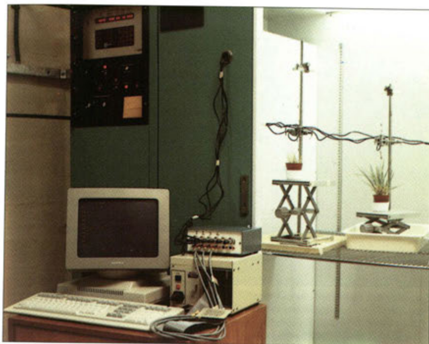
Figure 6. Two LVDT devices within a controlled environmental cabinet also showing attached data logger and visual display unit.
