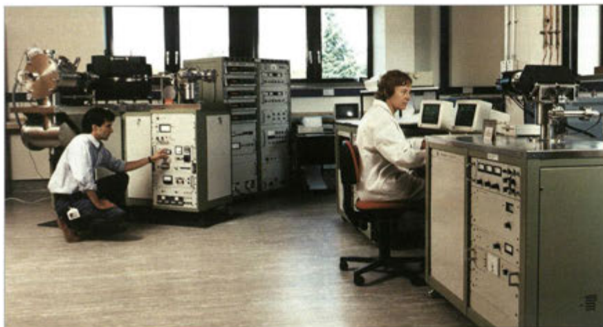
Measurement of stable isotopes of inorganic and organic elements by mass spectrometry
