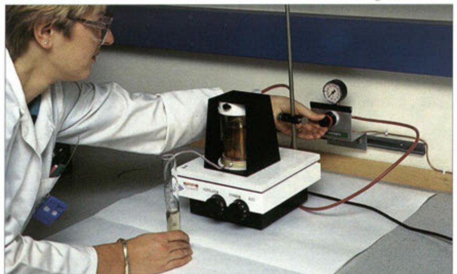
Figure 2. Ultrafiltration equipment used to determine the size distribution of P from soil solutions
