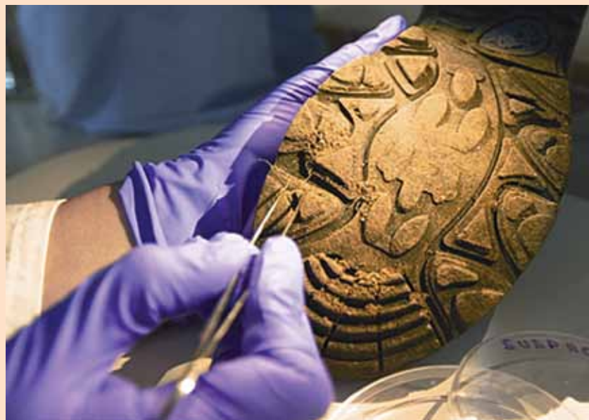
Figure 11 Soil forensic sampling of footwear sample
