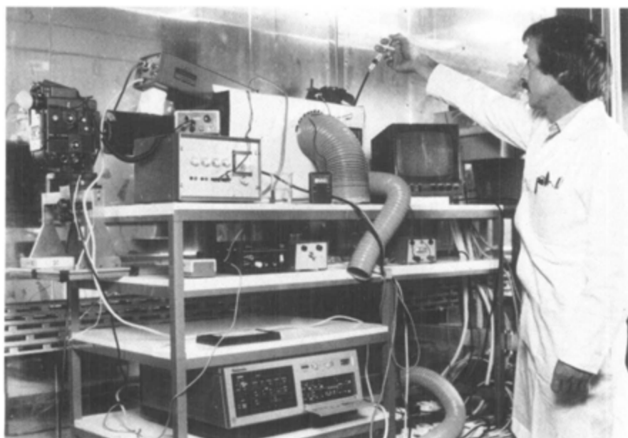
Time lapse cine and video equipment filming and monitoring potato growth.
