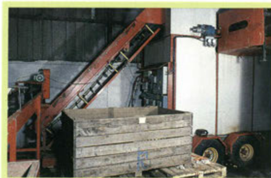
Figure 1 Continuous hot water treatment equipment: prewashed tubers being fed to hot water tank.
