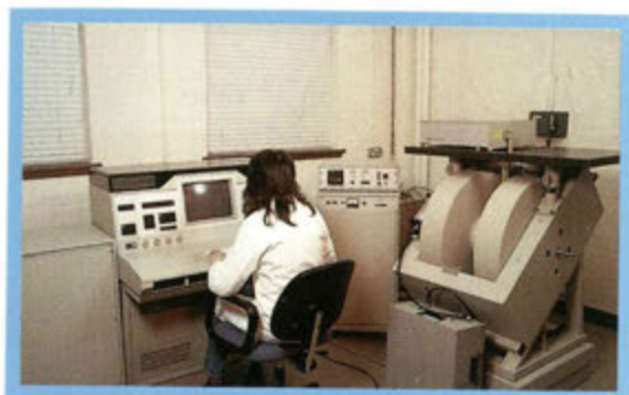
Figure 3 The Bruker ESP300E X-band EPR spectrometer at SCRI.
