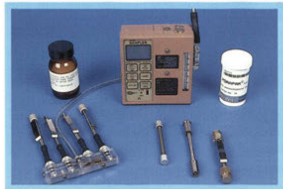
Figure 6 Field sampling pump and manifold.
