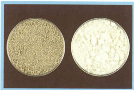
Figure 3 Delignification of barley straw with sodium peroxymonosulphate. Intact straw (left) and delignified straw (right).
