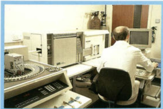
Figure 1 Automated thermal desorption and volatile analysis system.
