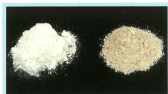
Figure 4 Effect of ozone on the delignification and bleaching of barley straw.
