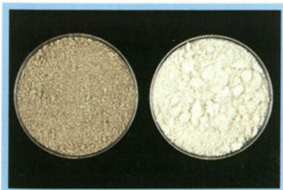
Figure 4 Loss of colour of barley straw after perborate treatment (l. untreated, r. treated).
