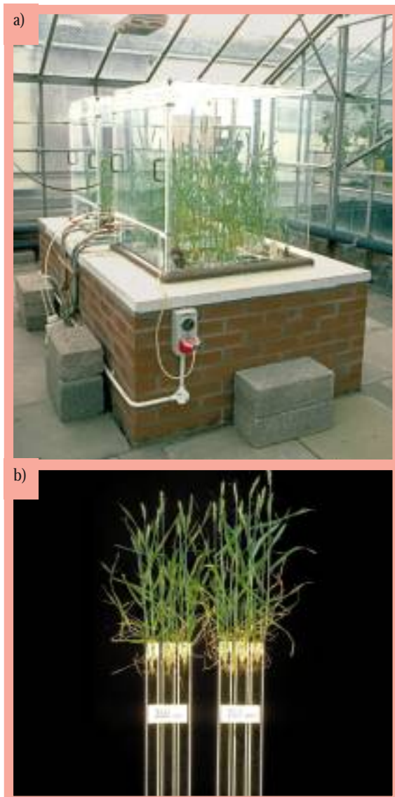
Figure 1 (a) Facility for growing plants at different CO 2 concentrations; containers filled with soil are surrounded by a cooling system in the brick base. (b) Soil containers (front cover removed) with spring wheat plants grown at 350 and 700 μmol CO 2 mol -1 for 87 days.
