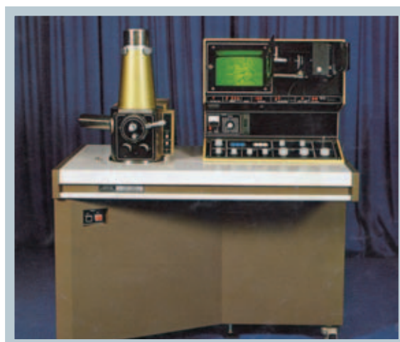
Figure 11 Jeol T 200 scanning electron microscope (1980 – present).
