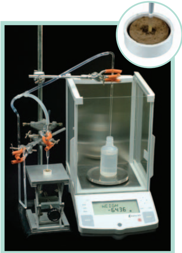
Figure 3 Device that allows the direct measurement of water transport properties of soil and repellency, at hitherto unattainable spatial scales.
