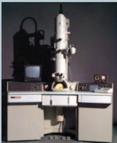
Figure 12 Jeol 1200 EX electron microscope ( 1985 – present).
