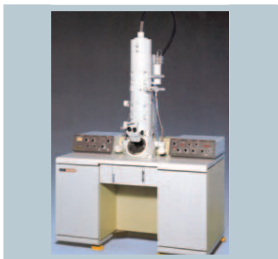
Figure 10 Jeol 100 S electron microscope (1980 – 1997).
