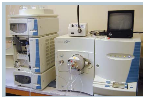
ThermoQuest LCQ-DECA LC-MS system.
