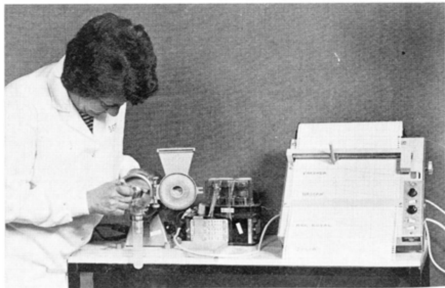
Milling energy apparatus and chart recorder being used to estimate grain hardness in barley as a measure of malting quality.
