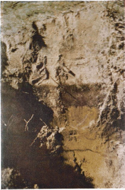
1. Blown sand above podzol with iron pan. Note (i) the series of buried A_1 horizons; (ii) the fairly well-developed A_2 horizon; (iii) the iron pan; and (iv) the humus bands in the B_2 and B_3 horizons.
