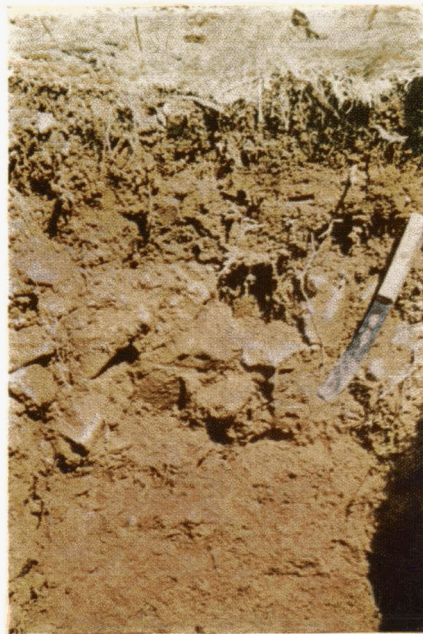
4. Darleith Association, Darleith series. Note the freely drained B_2 horizon with numerous stones, resting on shattered rock.
