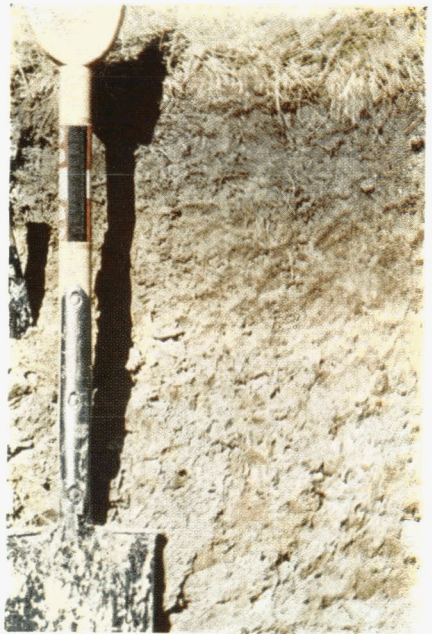
8. Ettrick Association, Ettrick series. Note the strongly gleyed B_{2g} and B_{3g} horizons.
