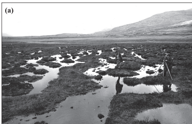
Figure 5(a) Theodolite being levelled at a survey point; (b) Sampling of a peat core at a survey point using a 'Russian Sampler'
