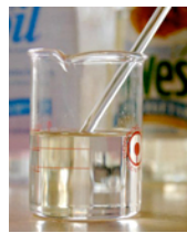
Figure 3. Pyrex rod immersed in RI matched oil solution. Edges of rod are invisible and solution is transparent
