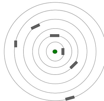
Figure 5- Aerial view of microcosm set up. Grey rectangles represent the blotting paper on which carbon will be captured. The blotting paper is attached to metal strips to keep them upright. The green dot represents the Rhizon sampler through which the carbon is pumped.
