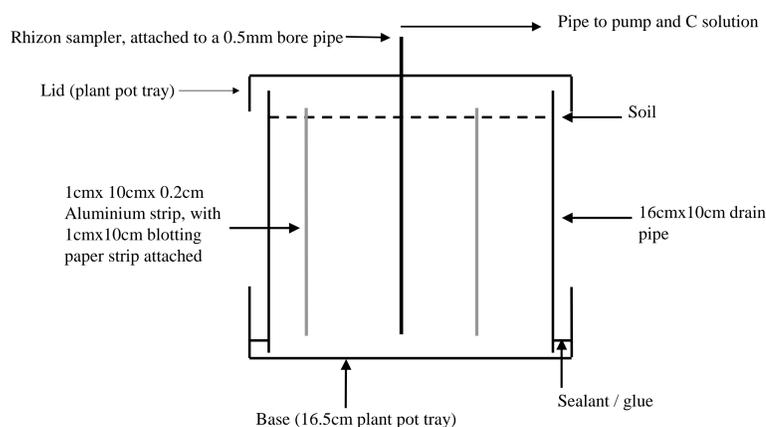
Figure 3- Microcosm set up
