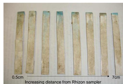
Figure 6- Blotting paper removed from microcosm after 12 hours of running dye through the soil system. Blotting paper on the left was closest to the Rhizon sampler.
