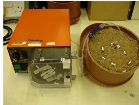
Figure 4- Microcosm and pump set up
