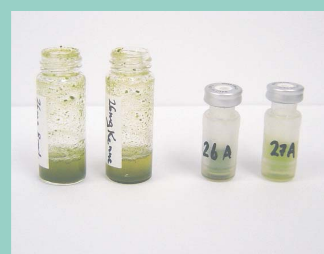
Dried tissues are milled, extracted in acidified methanol, and lyophilised prior to screening in high-throughput assays
