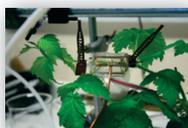
Figure 2 Copper support frame/ film close around plant stem and flushed out with filtered air.
