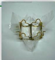
Figure 1 Sampling Enclosure - Copper support frames with PET film attached
