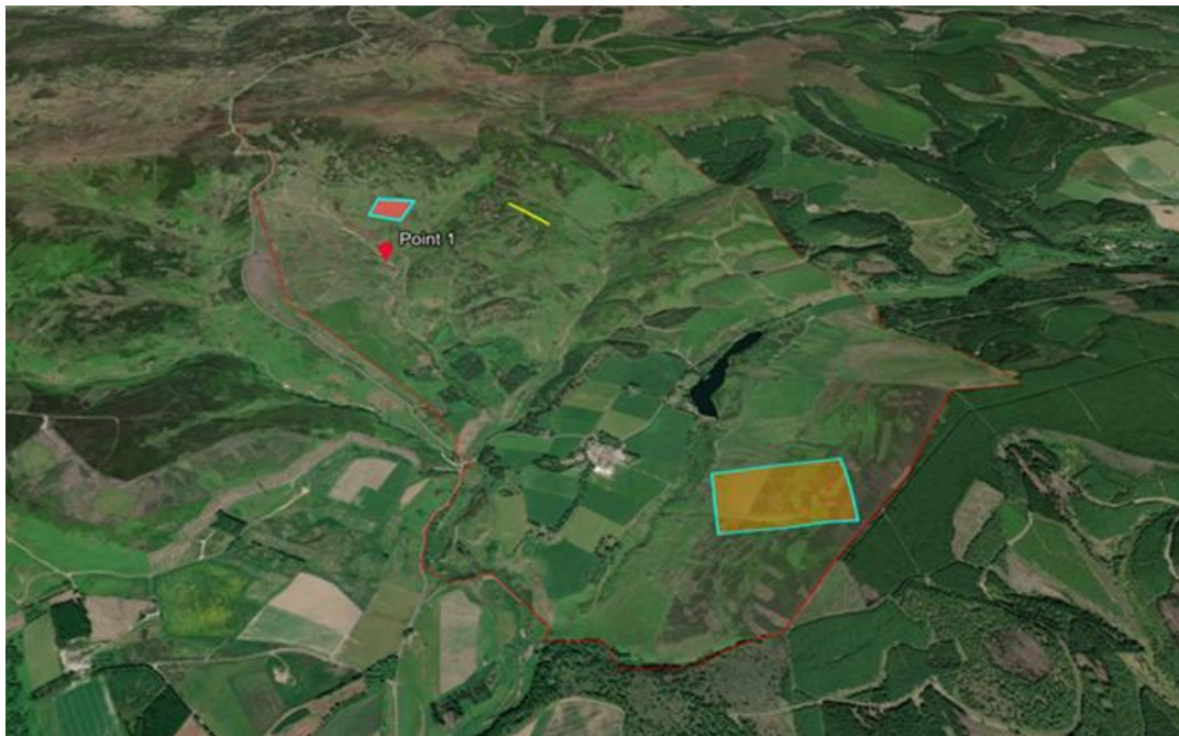
Figure 3: Example of how to make the selection of ecosystem services in the area of interest using polygon, punctual and linear elements in ArcGIS Earth.
