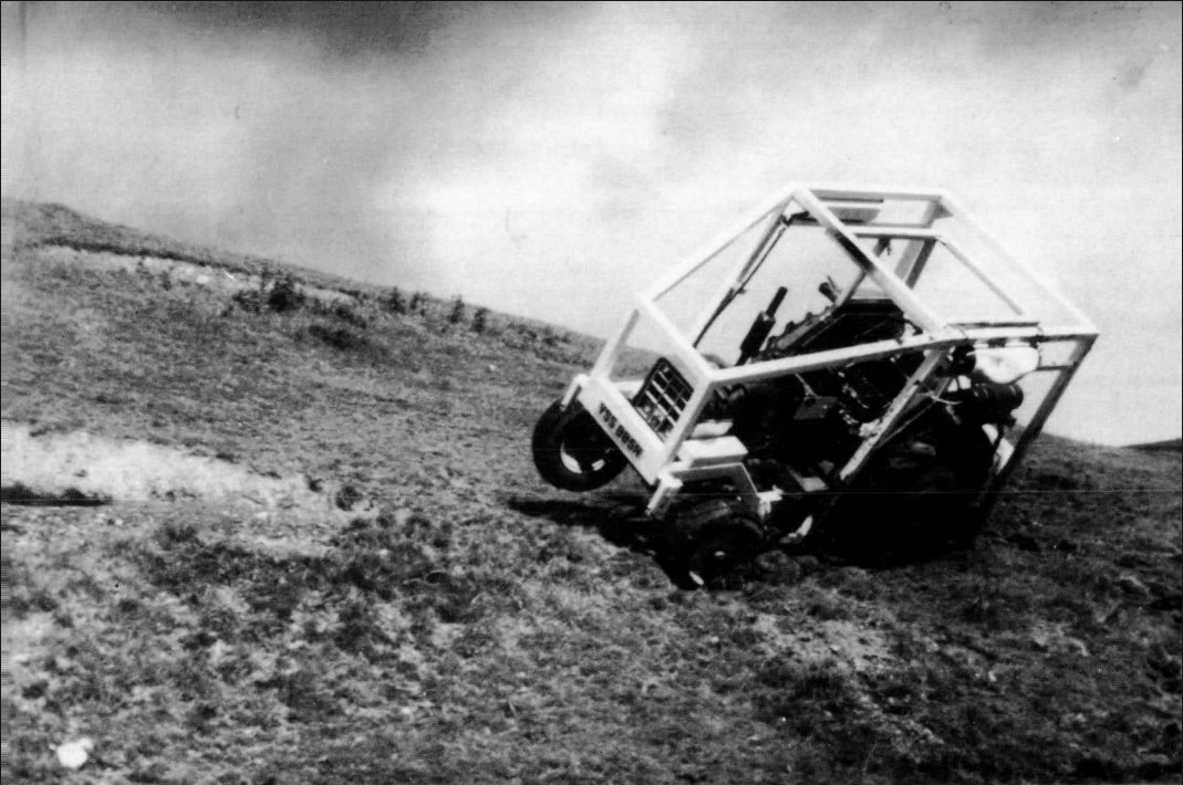
Plate 2 GRADIENT. A tractor, suitably modified for experimental work on stability, overturning on a slope when the angle of stability is suddenly exceeded due to a local slope irregularity. The difficulties of producing firm figures for slope limits is graphically illustrated. Photo: Scottish Institute of Agricultural Engineering
