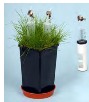
Figure 1: A mix of Agrostis capillaris and Festuca rubra growing within a pot containing two plant free soil cores. To the right of the pot is a core illustrating the mesh windows.
